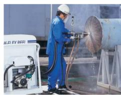
Inner surface cleaning of heat exchanger tubes by Flex
