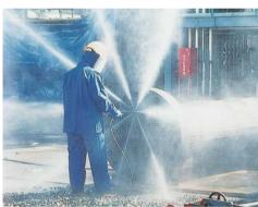
Cleaning of heat exchanger with Lance Nozzle.
